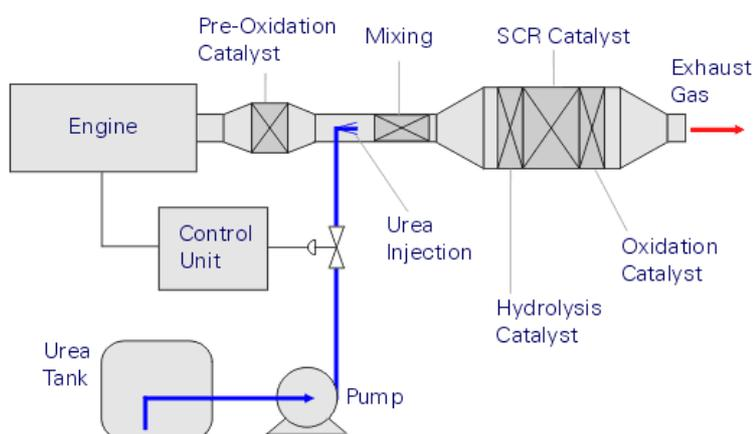
Selective catalytic reduction (SCR) is a technology that is starting to be seen on- highway, especially in Europe.
