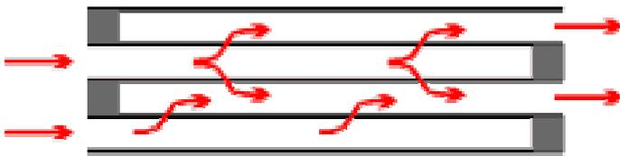
The exhaust gases actually flow through the porous walls of the material, depositing the particulate and leaving the exhaust gases clean.
