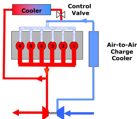
NO<sub>x</sub> is formed at very high temperatures within the engine's cylinder. A small proportion of exhaust gas can be cooled and introduced into the cylinder. As exhaust gas is high in water vapour (a by-product of the combustion process), this will act to cool the combustion and reduce NO<sub>x</sub> formation.
