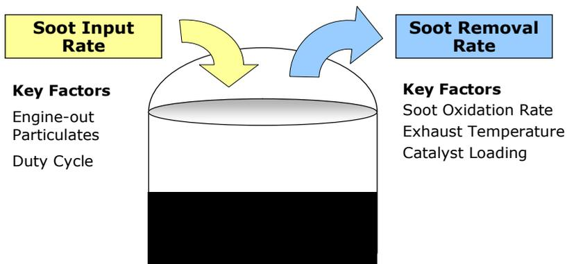
As the diesel particulate cleans the particulate matter from the exhaust gases, soot will start to accumulate in the filter. This needs to be cleaned out through a process called “regeneration”. The rate at which the filter fills depends on how clean the engine is and it is certainly desirable to make the particulate output of the engine as low as possible. The operating cycle of the machine also has some effect on the rate of soot accumulation.
