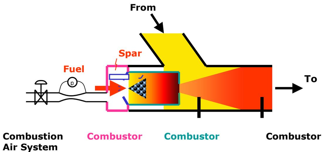
High temperature regeneration is an occasional process that is used to burn off the accumulated soot after a few hours of operation. There are several different methods, but the one preferred by Perkins, for engines over 130kW, is to use a burner in the exhaust stream, which heats the exhaust gases to over 600 °C, directly oxidising the accumulated soot in a well controlled manner.
