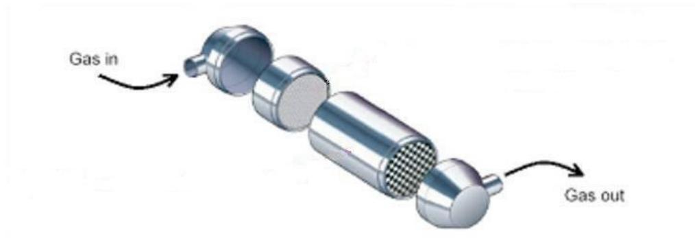
For low temperature regeneration, a catalyst of precious metal helps create  $\text{NO}_2$  in the exhaust gas which oxidises carbon at temperatures of around  $250\text{ }^\circ\text{C}$  or higher.
